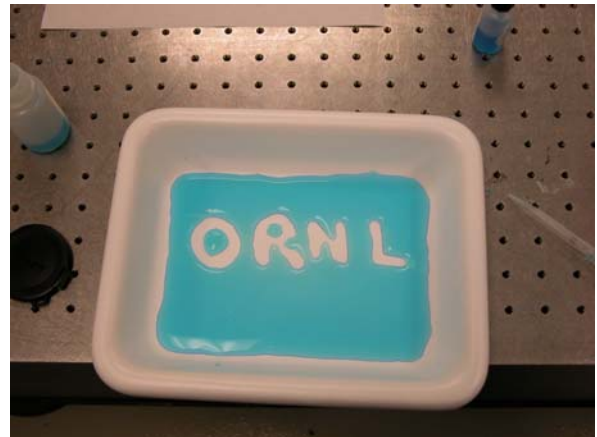
SH coated areas spell out "ORNL" by dramatically repelling water.
