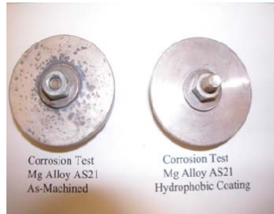
The above image is an example of using SH powder coatings as corrosion inhibitors. The magnesium (Mg) part on the right was coated with SH powder, while the Mg part on the left was not coated. Both parts were subjected to the same corrosive (salt spray) conditions. The coated piece was completely protected, while the one on the left was not.
